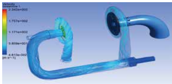
Horizontally back-to-back compression flow field analysis
