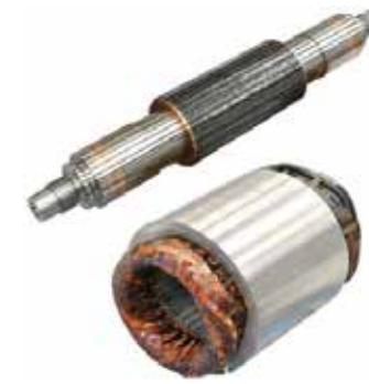
Permanent magnet motor
